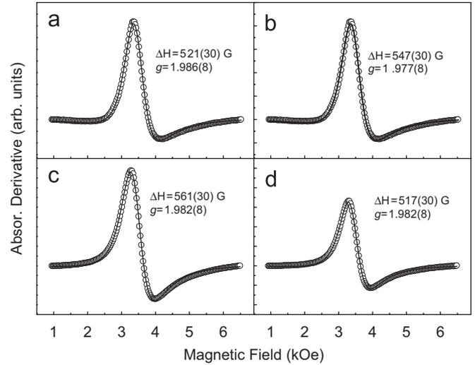
Fig. 2. ESR spectra at  $T = 300\text{ K}$  for (a)  $\text{GdInCu}_4$ , (b)  $\text{Gd}_{0.99}\text{Y}_{0.01}\text{InCu}_4$ , (c)  $\text{Gd}_{0.95}\text{Y}_{0.05}\text{InCu}_4$  and (d)  $\text{Gd}_{0.9}\text{Y}_{0.1}\text{InCu}_4$ . The solid lines are the fits to the Dysonian lineshape.
