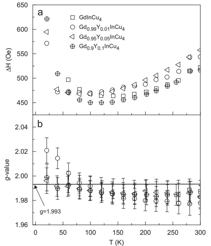
Fig. 3.  $T$ -dependence of the X-band ESR (a) linewidth,  $\Delta H$ , and (b)  $g$ -value of  $\text{Gd}^{3+}$  in  $\text{Gd}_{1-x}\text{Y}_x\text{InCu}_4$  ( $x = 0.01, 0.05$  and  $0.1$ ) single crystals.
