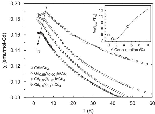
Fig. 1. Temperature dependence of the magnetic susceptibility at an applied field  $H = 1\text{ kOe}$  for the  $\text{Gd}_{1-x}\text{Y}_x\text{InCu}_4$ . Inset: The frustration parameter,  $f$ , as function of Ytrio concentration.
