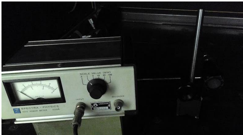
Figura 4 - Laser Machine Display Receiver da marca Spectra Physics.
