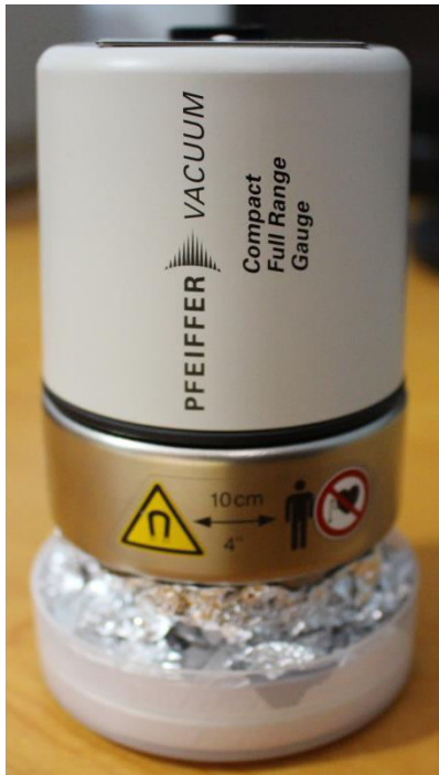
Fig 1. PKR 251 Compact FullRange™ Gauge, FPM Sealed da PFEIFFER VACUUM 1
