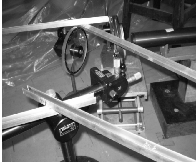
Figure 2: The Beam splitter and one of the spatial filters are fixed to other optical supporting elements.
