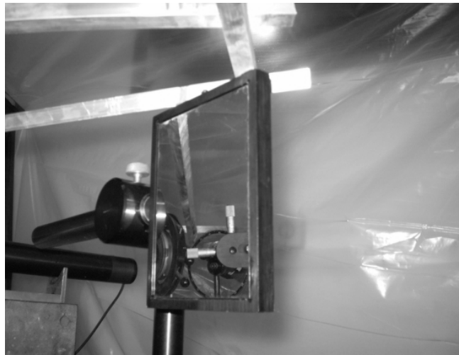
Figure 3: The glued bars on one of the plane mirrors, behind is the plastic film.
