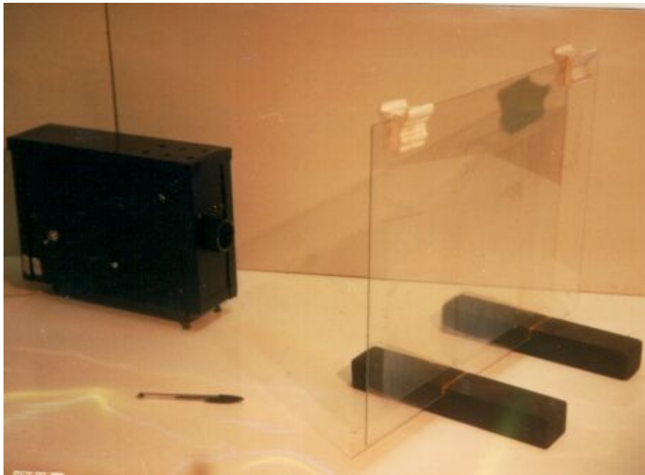
Fig.4: Holojector and screen, with size reference to a pen.
