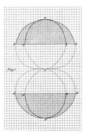
If, however, as with the multiplier of a tangent galvanometer, a rectangular cross-section is preferred, for which only the ratio of the two sides of the rectangle is to be determined, the following equation results for the former case, where the multiplier turns are circular, if the radius of the cylindrical space to be left free for the needle is set equal to 1 and the side of the rectangle parallel to the radius is denoted by a and the side perpendicular to it by 2b:
