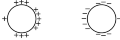
Figure 8.4: Qualitative distribution of surface charges for two parallel wires in the plane z = 0 .
