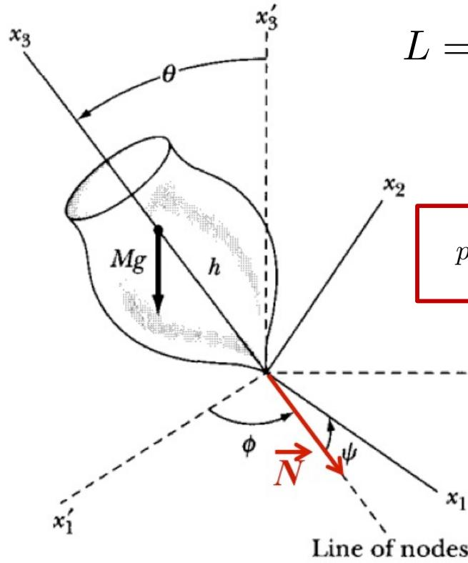
$$L = \frac{I_1}{2} \left( \dot{\theta}^2 + \dot{\phi}^2 \sin^2 \theta \right) + \frac{I_3}{2} \left( \dot{\psi} + \dot{\phi} \cos \theta \right)^2 - Mgh \cos \theta$$
