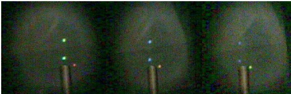
Fig. 4. (2.5 Mb) Parallax and color change for three point objects (see video). a) left view b) center view c) right view
