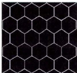
Figure 1: Scheme of the array of hexagons used as a mask transparency for observation of the Talbot images. The lateral side of each hexagon was 250 \mu\text{m} and the total area of the array was a circular spot of about 5 mm of diameter. The mask was printed in a photo-lithe.
