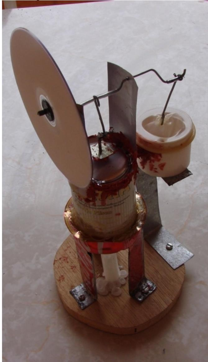
Figura 13 – Motor Stirling
