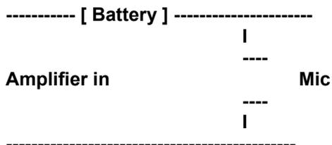
This circuit works if the microphone preamplifier passes through some small DC current and is not bothered by it. This quite often the case but not always. Normally direct current from the battery has no influence on the preamp, as the preamp is only amplifying alternating currents.
