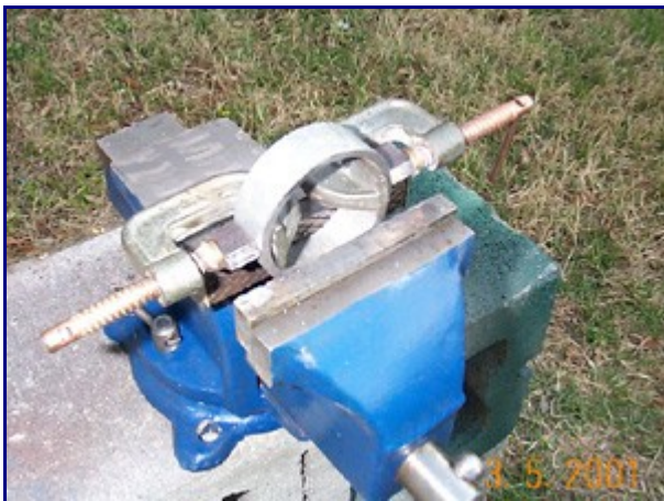
Gimbal ring ready for welding
