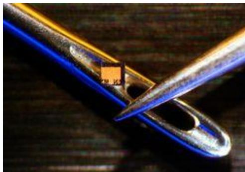
Image of the actual laser diode chip (shown on the eye of a needle for scale) contained within the package shown in the above image.
