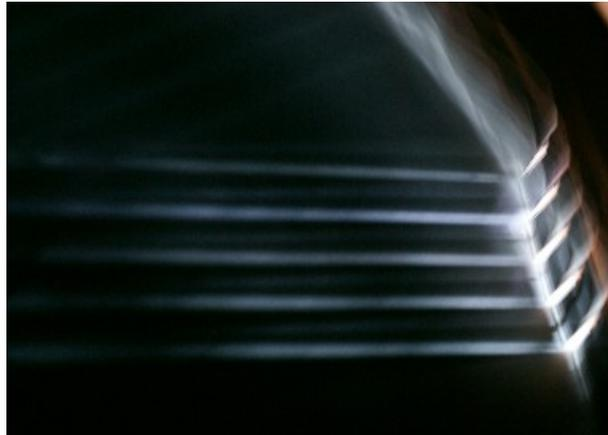
Figura 6. Raios obtidos com as fendas
