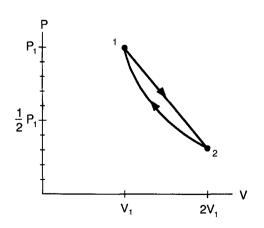
Fig. 2. A reversible cycle using a straight path and an adiabatic.
