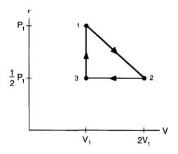
Fig. 1. A PV diagram of a reversible cycle.
