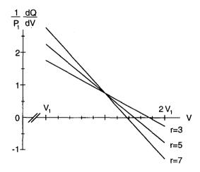
Fig. 5. Change in heat as a function of volume for the path  $1\rightarrow 2$  of Fig. 1; r=number of degrees of freedom.
