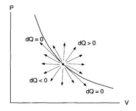
Fig. 7. Whether heat enters or leaves a system depends on the path taken relative to the unique adiabatic through each point of a PV diagram.
