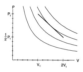
Fig. 3. Comparison of path  $1\rightarrow 2$  of Fig. 1 and various isotherms. Only one isotherm is tangent to the path and it gives the maximum temperature attained.
