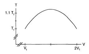
Fig. 4. Temperature along path  $1\rightarrow 2$  of Fig. 1. The maximum temperature is  $(9/8)T_1$  at volume  $(3/2)V_1$ .
