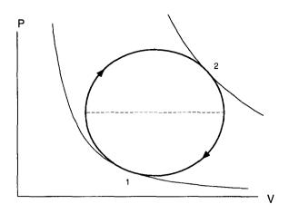
Fig. 9. A symmetrical cycle. The adiabatic curves tangent at points 1 and 2 indicate where the heat changes sign.
