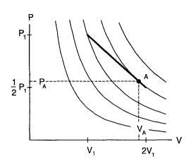
Fig. 8. The sloping path of Fig. 1 and various r=3 adiabatics. The point  $(P_A, V_A)$  is also shown.
