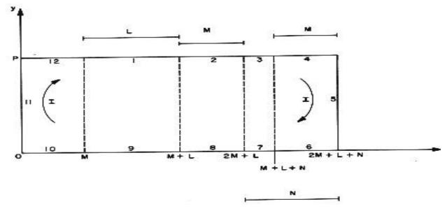
Fig. 1.- Electrical circuit with steady current I. The bridge is represented by 1 and the remaining circuit (The support) by 2 to 12
