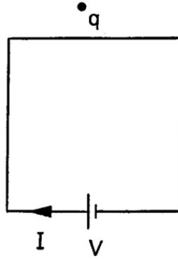
Fig. 4. Square circuit of side  $l$  made of a cylindrical wire of radius  $a \ll l$ , with a point charge close to the middle of one of its sides.
