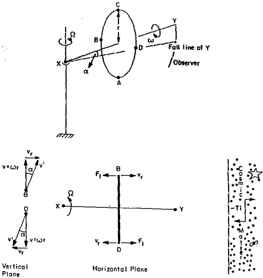
Fig. 5: Precession torque  $T_l = 2rF_l$  of flywheel
