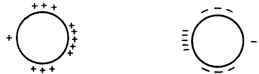
Figure 4. Qualitative distribution of surface charges for the two parallel wires at z = 0 .
