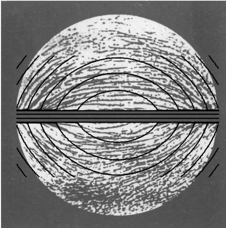
Experimental lines of electric field compared with theoretical calculations.
