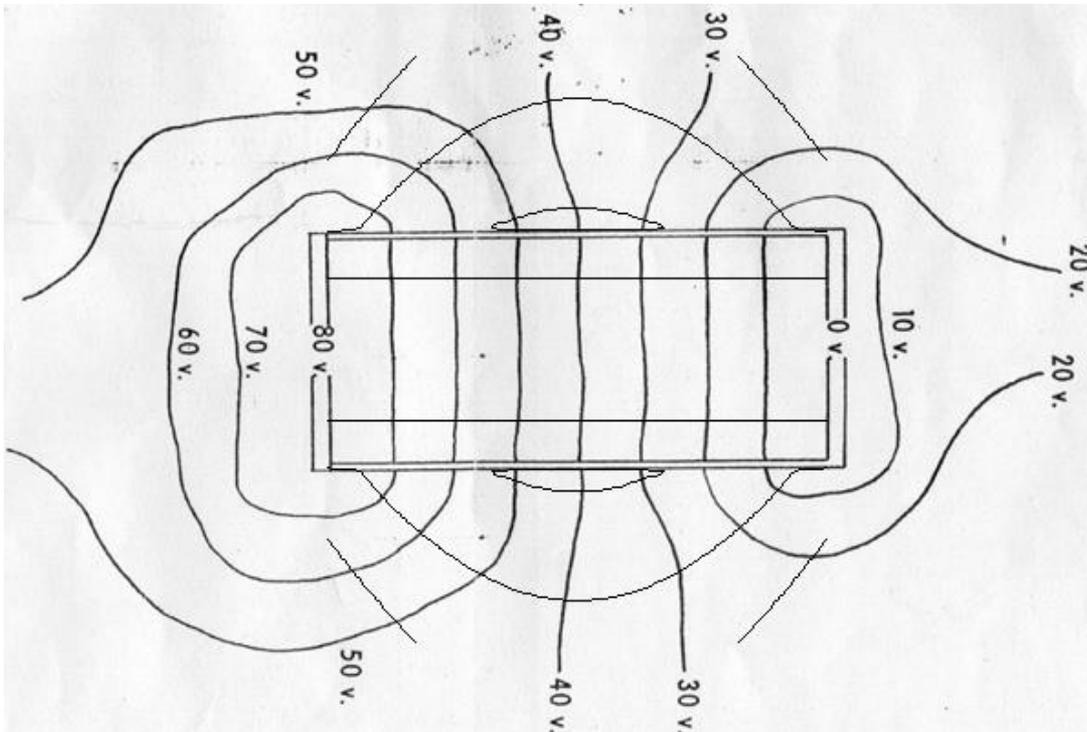
Experimental equipotential lines compared with calculated lines of electric field.
