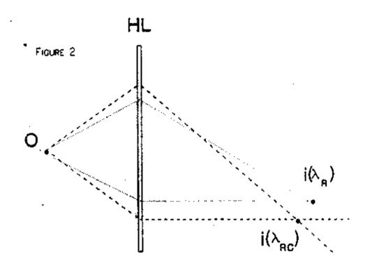
We assume for the moment to have the same wavelength  $\lambda R$  for reconstructing and registering the holographic lens. If we project an image on the screen from an objective whose optical center is located at point 0, and by assuming the approximation that the aperture of the
